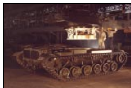
Turret married to hull on a Chrysler-built M60 during the Cold War
